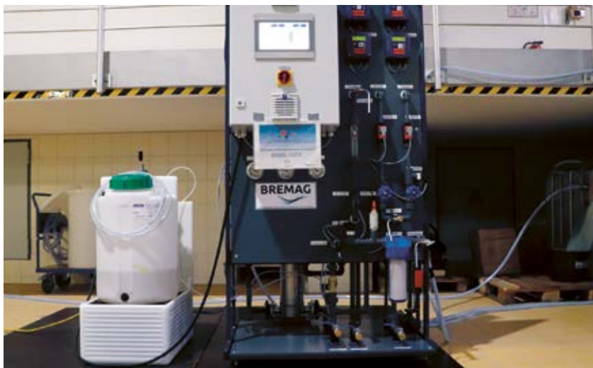
Pilot plant of low-pressure reverse osmosis at water works Berlin-Friedrichshagen (front and back view)
