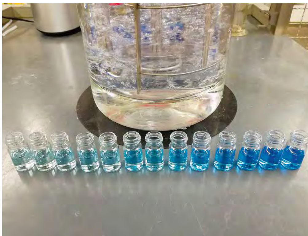
Quantification of soluted Ozone by using decolouration of Indigoblue
