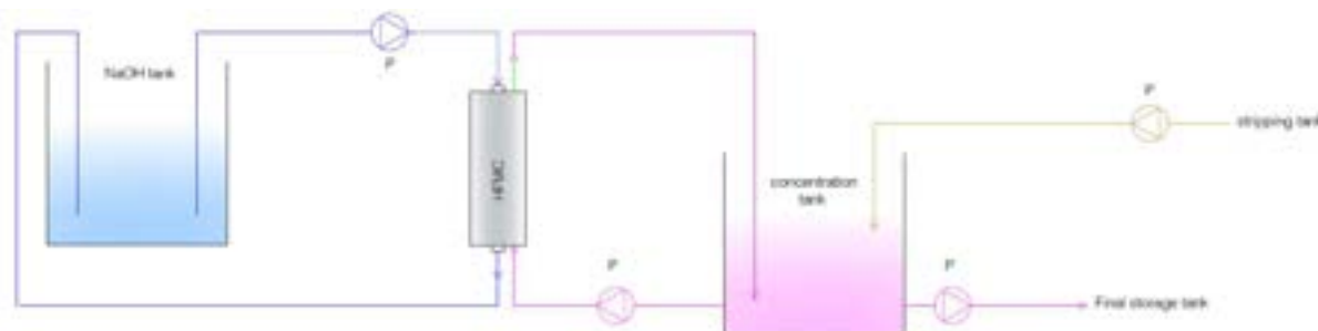
Figure 49 Simplified diagramme showing the concentration unit implemented in Yverdon
