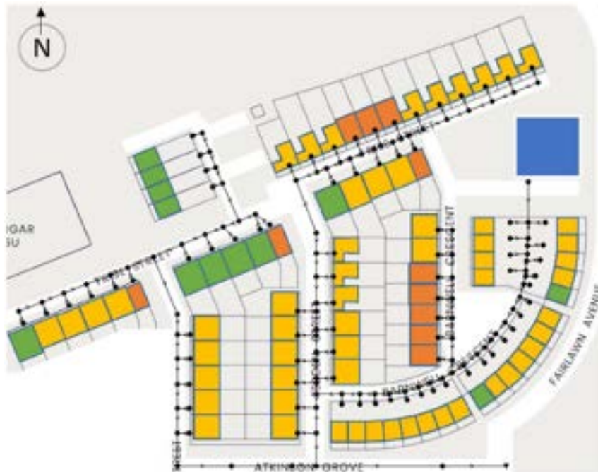
Figure 78 Sewer network overlaid onto housing map (SWMM)
