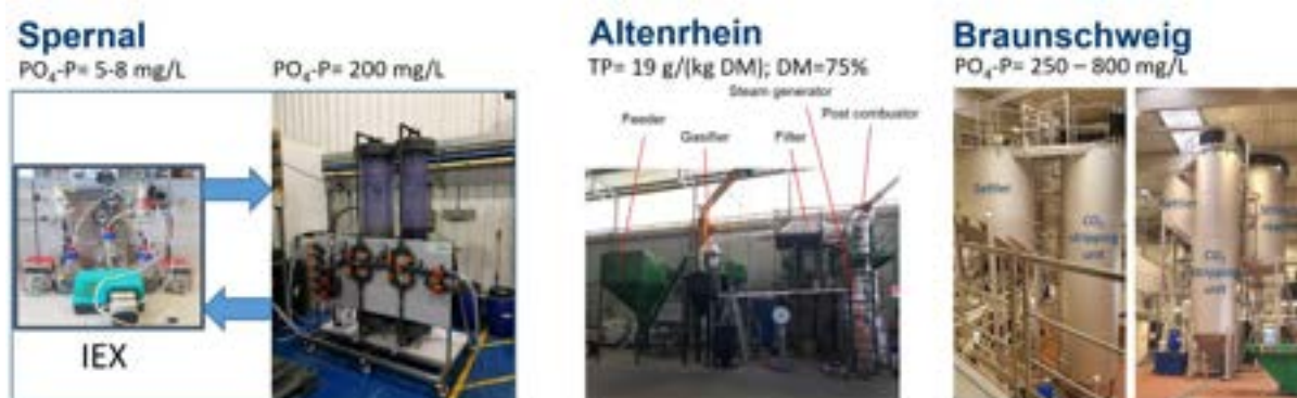
Figure 95 Phosphorus recovery technologies in NexGen with feed concentrations or contents
