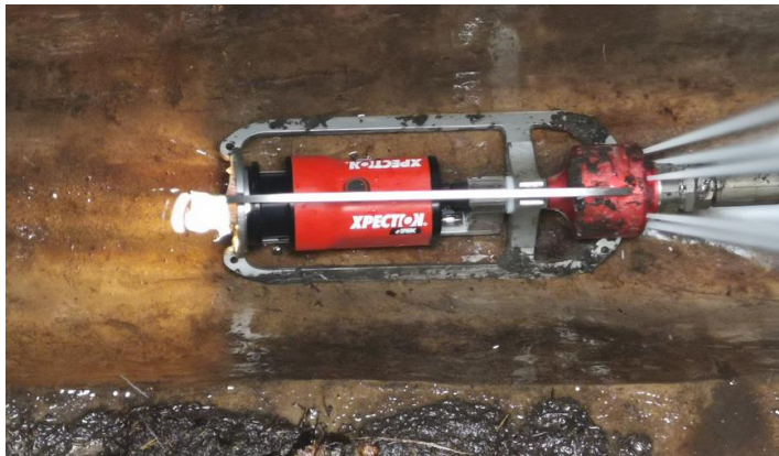
Figure 22: A iPEK XPECTION device for smart sewer cleaning.
