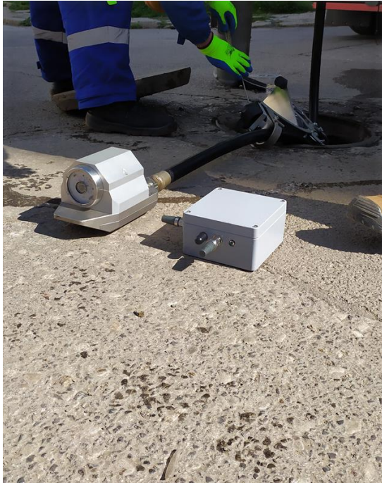
Figure 23: A iPEK XPECTION device for smart sewer cleaning in usage in Sofia.
