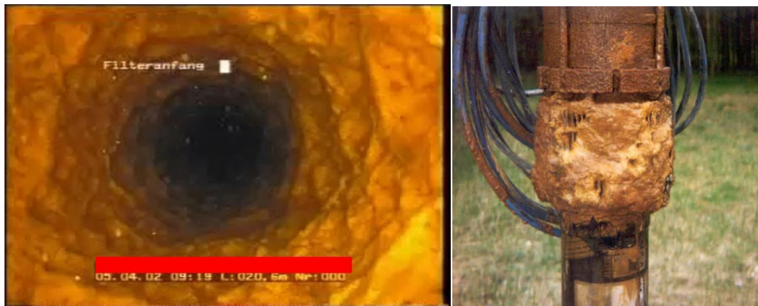
Figure 5: left: clogged well, ochre deposits inside the screen; right: clogged pump, ochre deposits at the pump intake, both ©BWB
