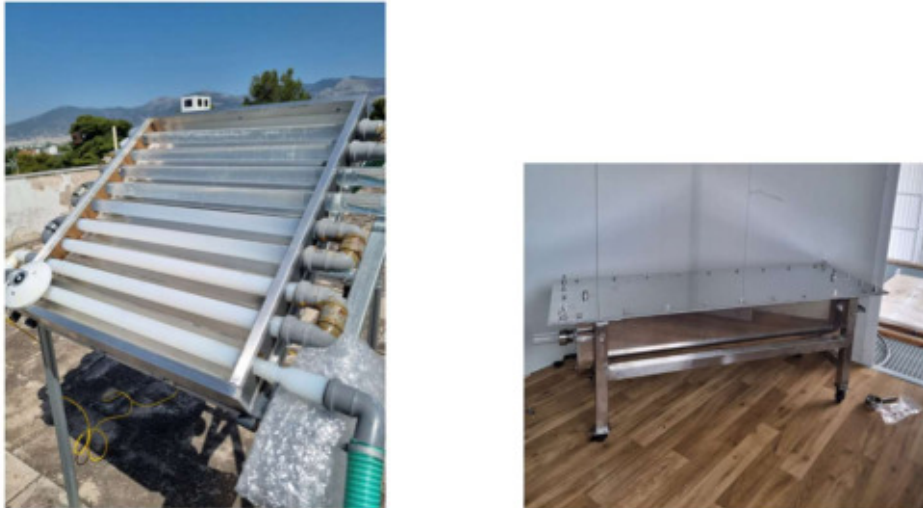
Figure 49. CS4 photocatalytic reactor.
