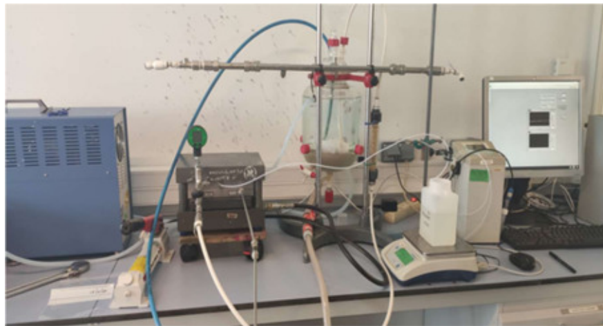
Figure 11. Reverse Osmosis laboratory experimental set-up.
