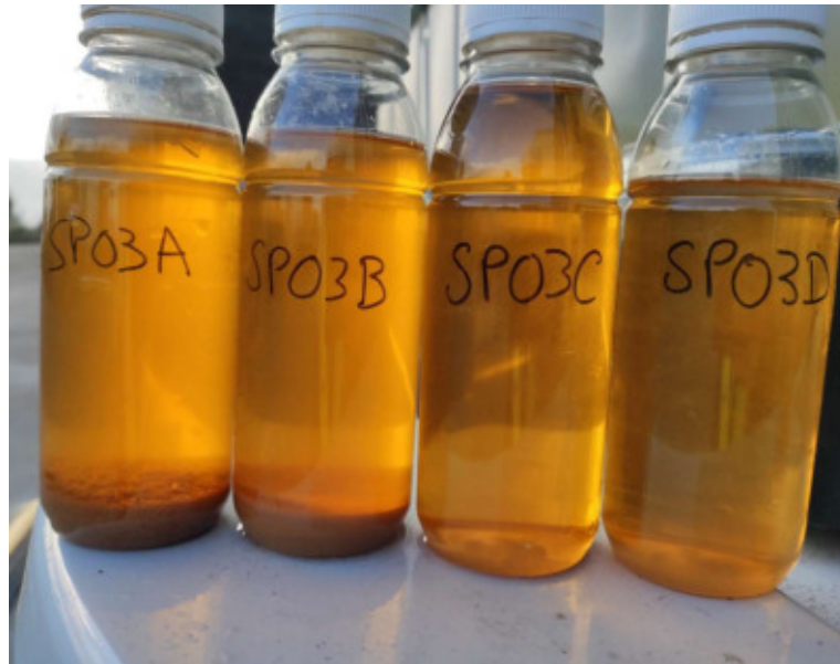
Figure 99. Samples collected from the different sections of the reactor A to D, from bottom to top.
