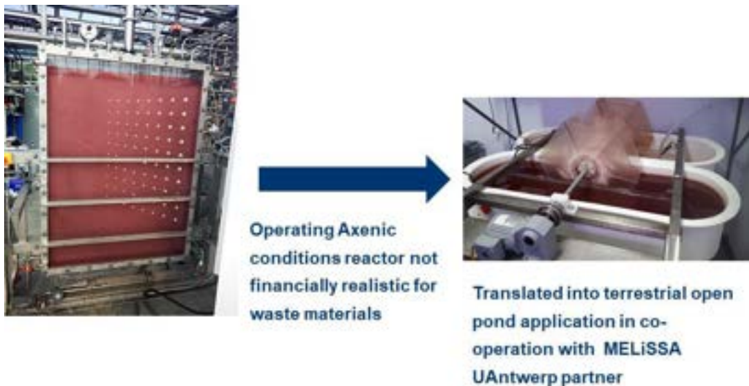
Figure 35 Pictures of the axenic MELiSSA purple bacteria reactor (Giurgiu et al. 2020)
