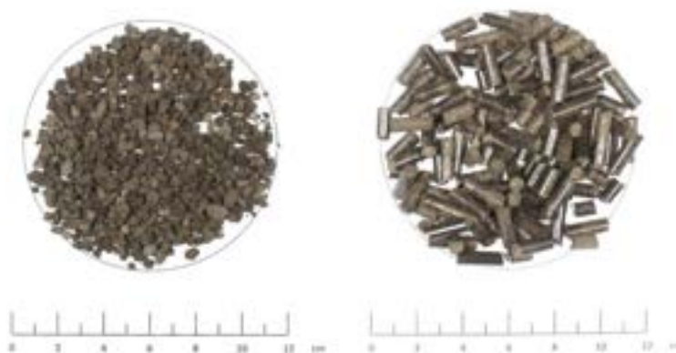
Figure 30 Left: feedstock before pelletising; right: pelletised sludge
