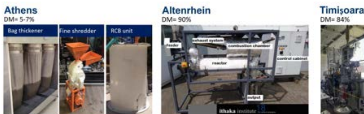
Figure 92 NextGen technologies for material recovery from sludge with dry matter (DM) contents of their inflow streams
