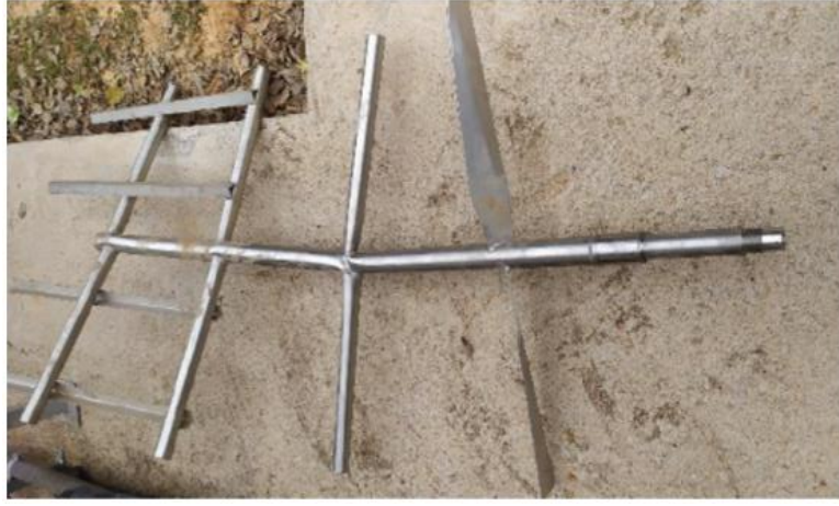
Figure 8 Left: Deformed mixing arm; middle: adjusted design of the mixing organ; right: new mixing organ
