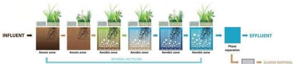
Figure 9: Scheme of a plant root enhanced IFAS (STOWA, 2017).
