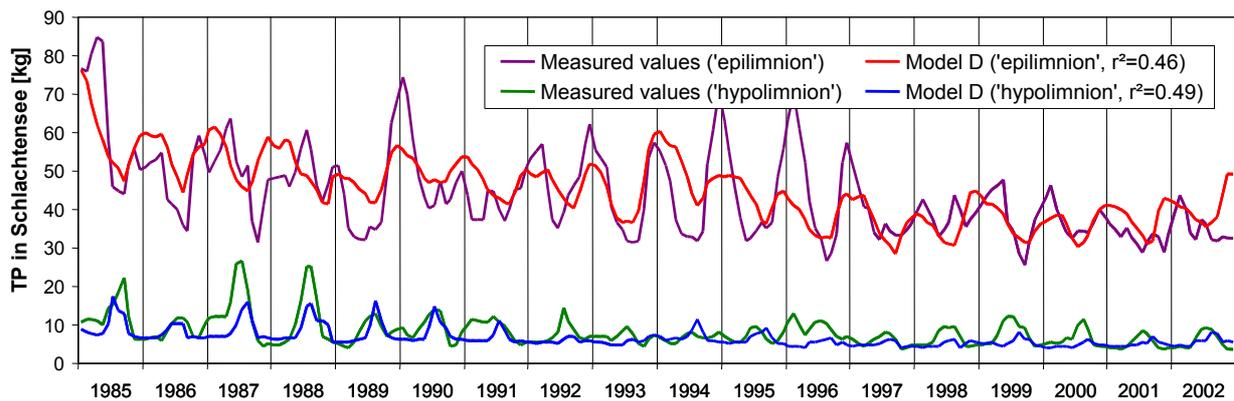
**Fig. 22.** P mass balance for Schlachtensee: results of Model D for the upper and the lower compartment [ $g P m^{-3}$ , monthly mean values]
