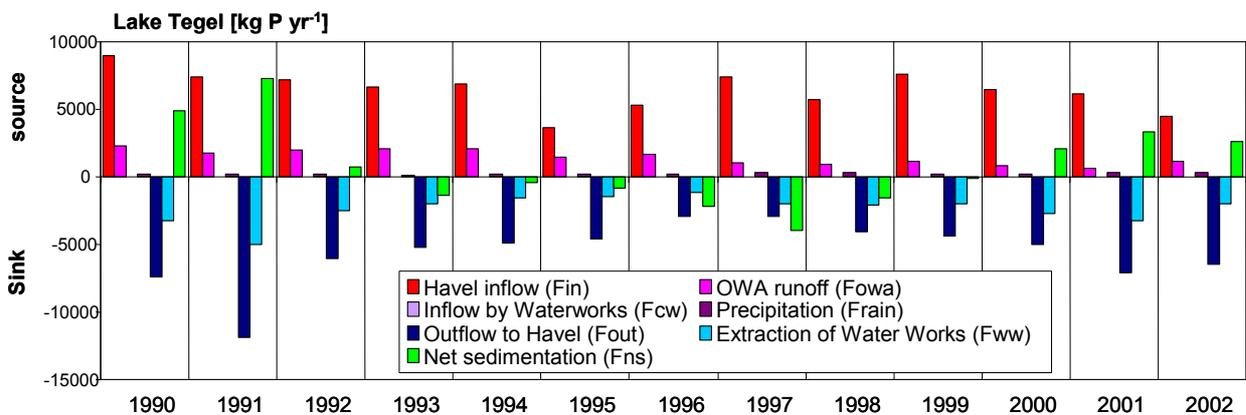
Fig. 28. P sources and sinks of Lake Tegel 1990-2002 [kg yr<sup>-1</sup>]
