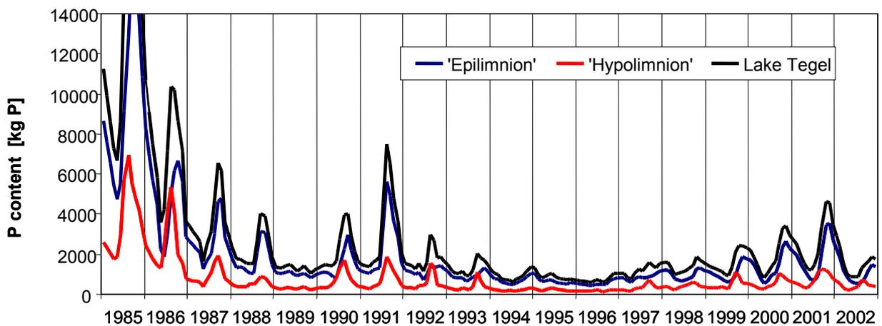
Fig. 27. P content in Lake Tegel, the upper (< 8m) and lower compartment (> 8m) [kg]
