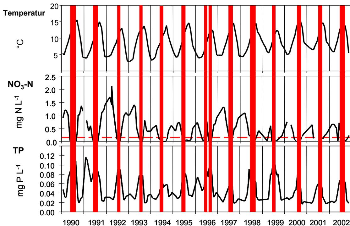
**Fig. 24.** Temperature, nitrat and phosphorus in 7 m depth in Schlachtensee
