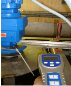
Figure 23: Experimental set-up for the G value measurement
