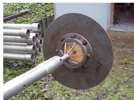
Figure 13: Packed flow meter [Wiacek 2003]
