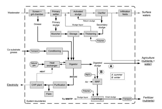
Figure 3: Scope of LCA study of wastewater treatment scheme in Braunschweig 2010 (secondary products are underlined)
