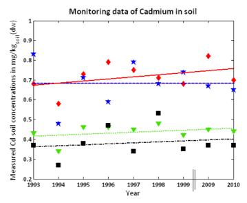
Figure 7: Monitoring data of different areas in Braunschweig irrigated with WWTP effluent and sludge
