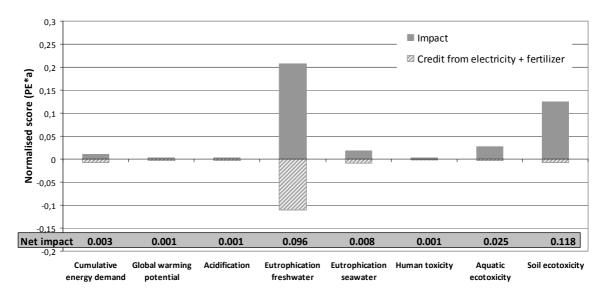
Figure 4: Normalised environmental profile of the Braunschweig wastewater scheme in relation to total environmental impacts in Germany
