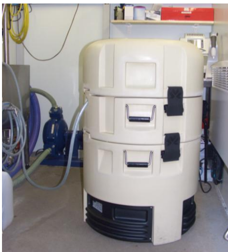
Figure 6. Bypass, autosampler, pump and probes for measurement of water quality in the container
