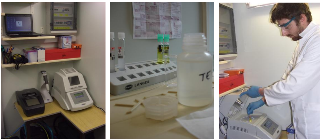
Figure 8. Laboratory instruments for sample analysis on site: pipette, thermostat and photometer.
