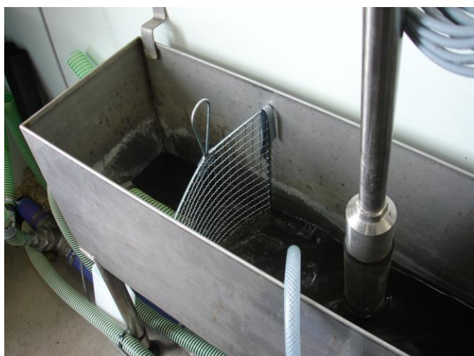
Figure 6. Bypass, autosampler, pump and probes for measurement of water quality in the container
