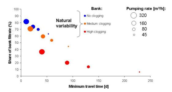
Figure 3 Process-driven simulation model (Bank Filtration Simulator): Impact of different pumping rates under uncertain clogging parameter (no clogging: no difference in hydraulic conductivity between aquifer and bank; medium clogging = 100 times lower hydraulic conductivity in bank than in aquifer; high clogging = 5000 times lower hydraulic conductivity in bank than in aquifer) on both, bank filtration share and minimum travel time.
