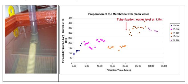
Figure 2 - Permeablity Tests with the membrane before and after the addition of an open-air tube on the permeate pipe
