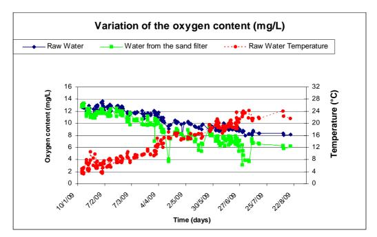
Figure 10 - Effect of temperature on the oxygen content
