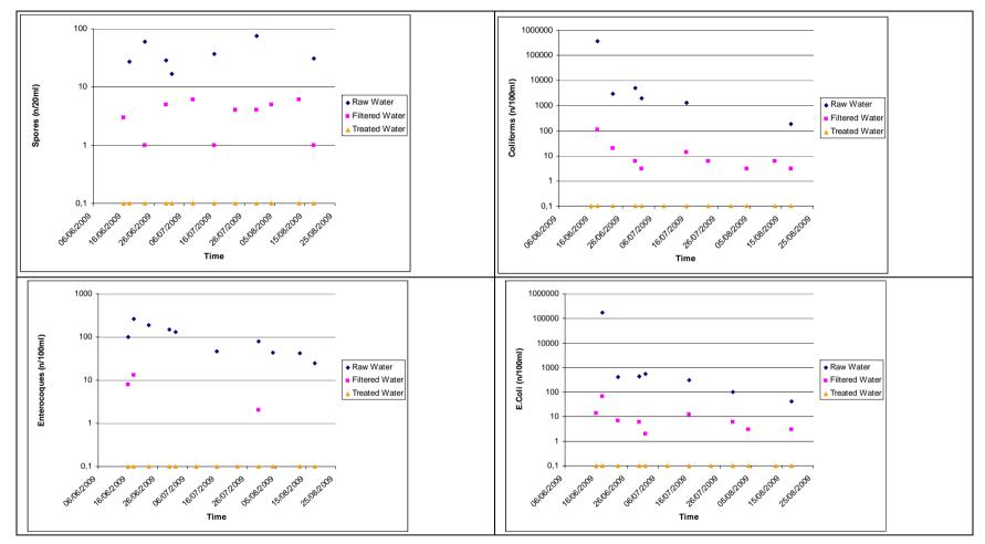
Figure 4 - Bacterial Analyses. Results for Spores, Coliforms, Enterocoques and E.Coli.
