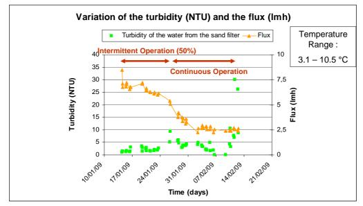
Figure 6 - Flux variation in regards to intermittent operation and turbidity feed
