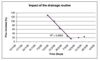
Figure 8 - Flux enhancement due to the drainage routine
