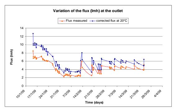
Figure 9 - Flux enhancement with a 20°C-correction
