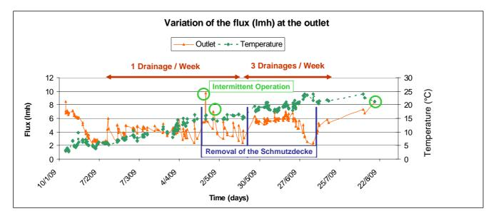
Figure 11 - Variation of the flux in function of the Operation and Maintenance conditions
