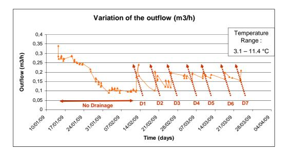
Figure 7 - Flux variation in regards to the drainage frequency
