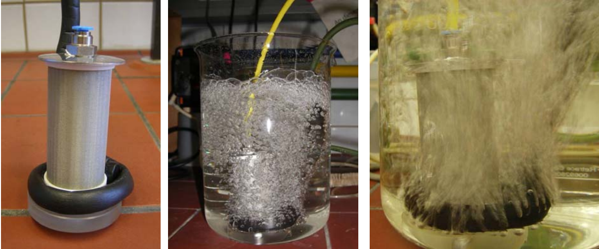
Figure 5: Steel filter used for the 1 μm filtration
