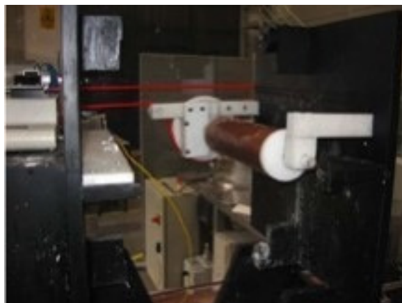
Figure 54. Picture of the electrospinning prototype designed and constructed by TTX
