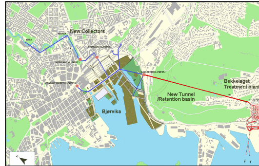
Midgardsormen, interceptors and retention basin
