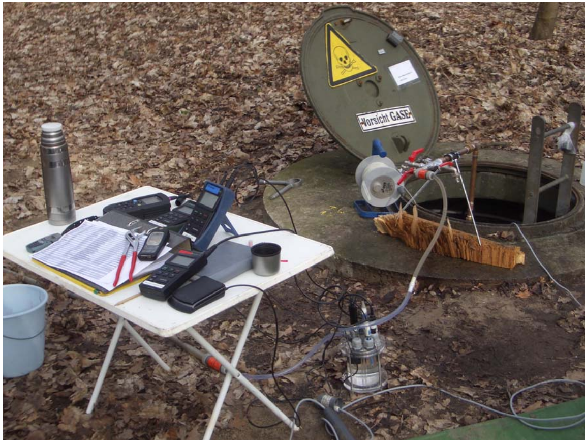
Figure 3-13: Sampling devices for the short term monitoring for microbiological and hydrochemical water sampling. Measuring system with flow-through cell for hydrochemical field parameters.
