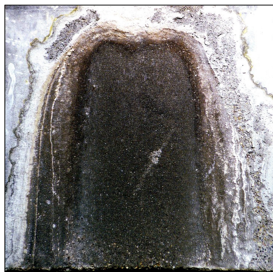
Optimized concrete 320kg BM: Z+FA+MS, w/b=0,42
