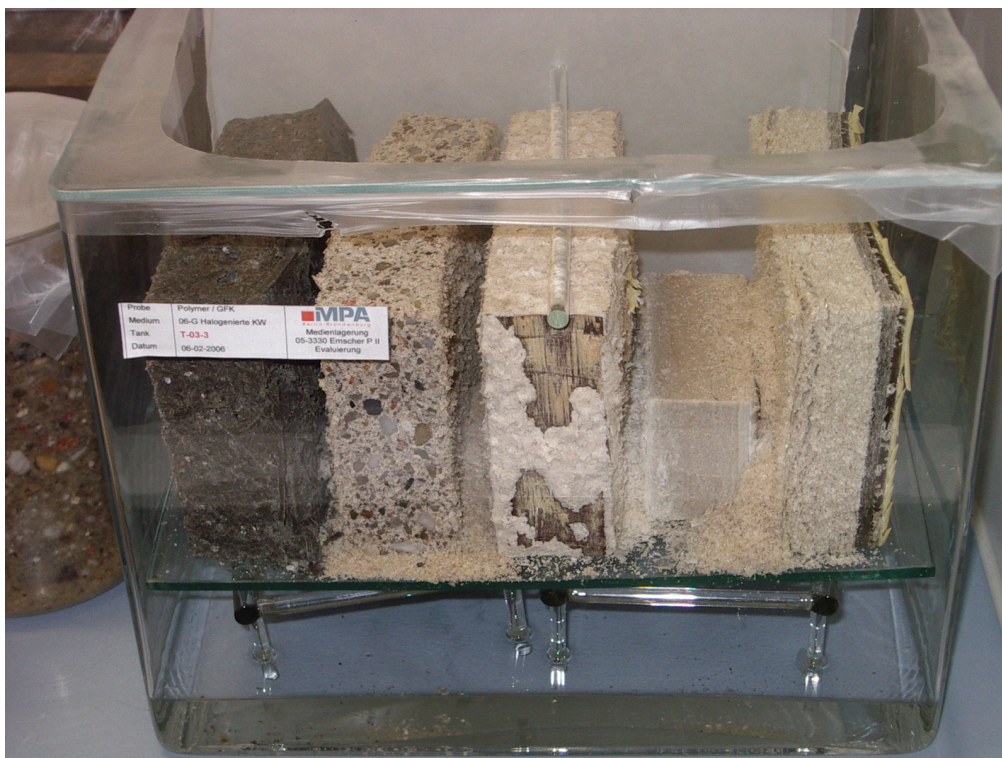
Figure 8: Various polymer concretes after 20 hours in the gas phase of halogenated hydrocarbons
