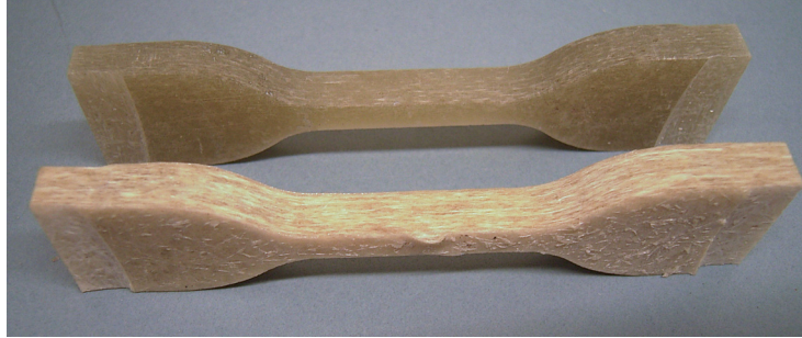
Figure 7: Front: GFK-specimen stored in halogenated hydrocarbons for 14 days. The plastic has dissolved, merely the glass fibres remain. Back: Specimen without loading for comparison
