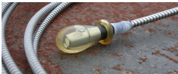
Figure 11: Prefabricated anchors with fixed pH sensors (arrows). Photo: BAM
