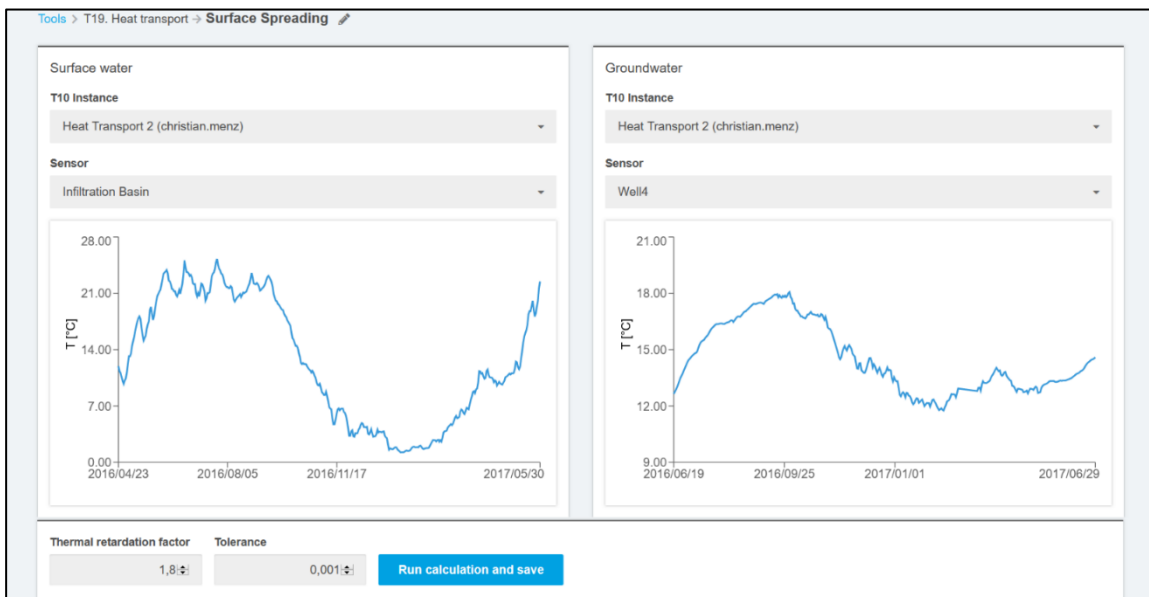
Figure 6. Screenshot of the Heat Transport Tool for hydraulic residence time assessment. Selection and display of input data
