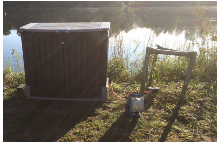
Figure 8. Sketch of sampling line for flow-through cytometry (left). Field box with sampling line next to the observation well SPA168 and infiltration basin 1+2 (right)
