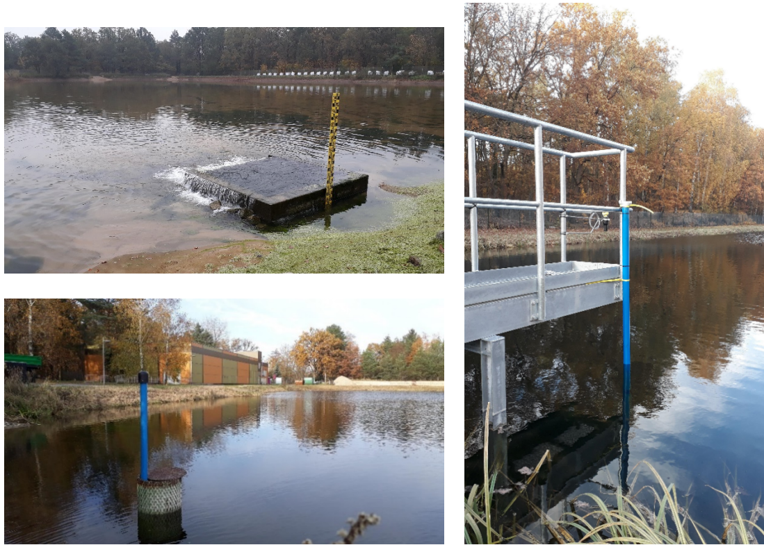
Figure 4. Manual water level meter (upper left) and installation of the online sensor devices at infiltration basin 1+2 (lower left) and basin 3 (right)
