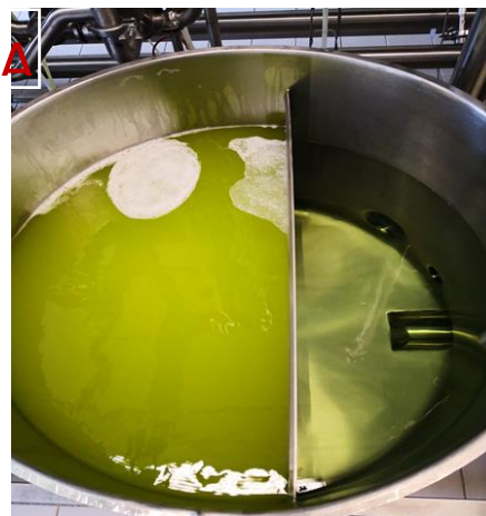
Fig. 38 Tank with the concentrated whey (a) and the purified stream (permeate)
