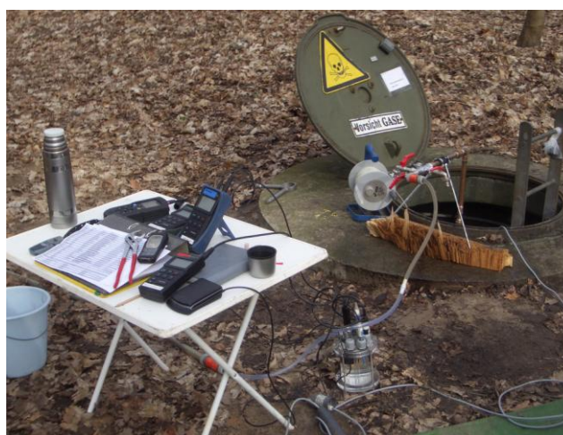
Fig. 3: Sampling devices for the short term monitoring for microbiological and hydro-chemical water sampling. Measuring system with flow-through cell for hydrochemical field parameters [FUB 2008]
