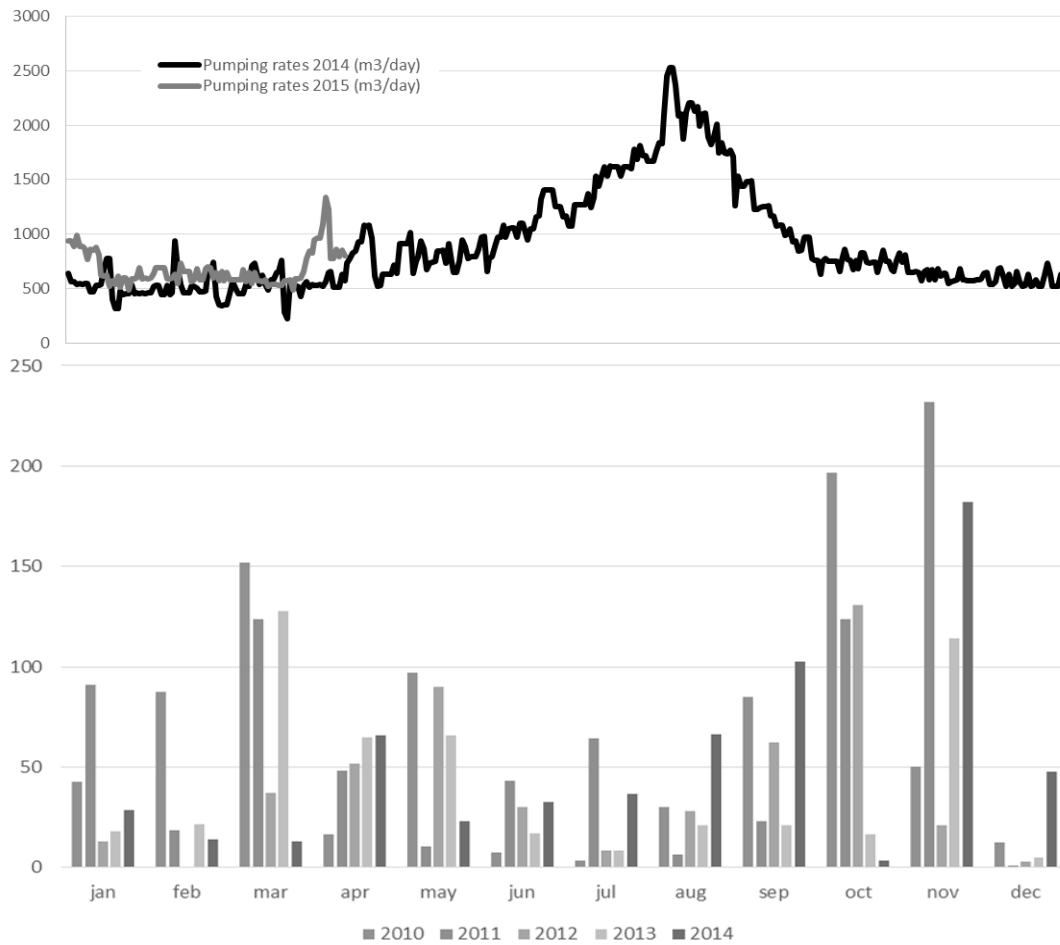
Figure 60 Daily pumping rates for 2014-2015 (top, data available until 12/4/2015) and rainfall for the period 2010-2015 (bottom, mm/month).
