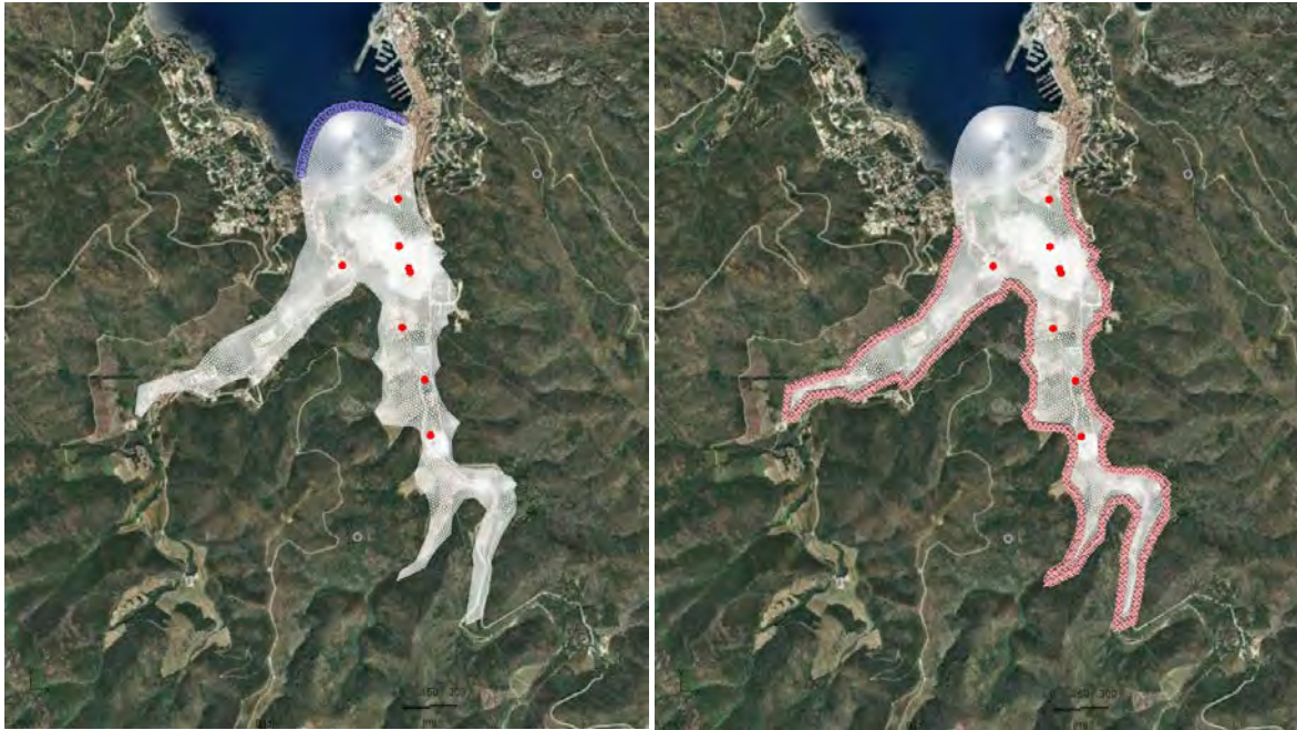
Figure 62 Boundary conditions: left: fixed heads with Dirichlet boundary condition (Sea level); right: hill slope inflow (Neumann boundary condition). Red dots: network of monitoring wells (Pz3,4,6,7 not shown)
