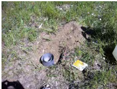
Figure 43 Infiltration tests conducted in river bed and soil at the recharge site.
