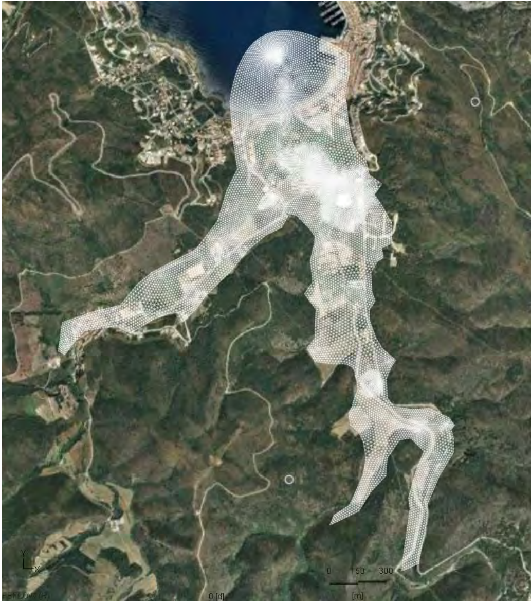
Figure 61 Finite Element discretization and model domain.
