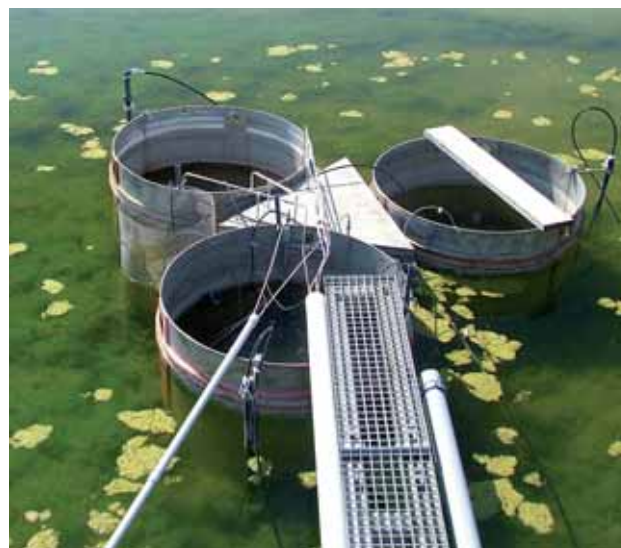
Picture 2 Enclosures for technical scale experiments on the UBA's Center for Aquatic Simulations, Berlin
