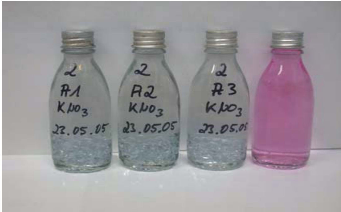
Figure 12: Screw cap tubes filled with sulfide reduced anoxic medium supplemented with \text{KNO}_3 . The pink bottle shows an example of oxidized medium.
